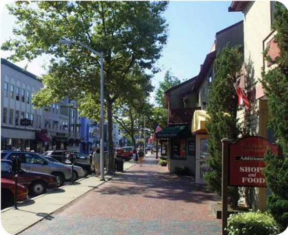
Figure 6.20 This sidewalk is wide enough and smooth to comply with ADA requirements.
